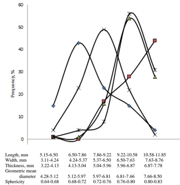
Fig. 3: Frequency distribution for the axial dimensions of coffee seed: ■, length; ▲, width; x, thickness; \*, geometric mean diameter; ◆, sphericity
