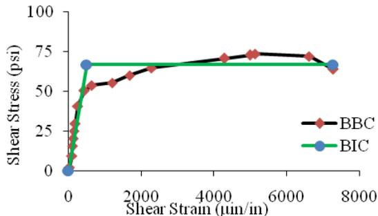
Fig 14: Bi-linear Idealized Curve (BIC) of double wythe shotcrete diagonal prism, (DWD\_1.5'')
