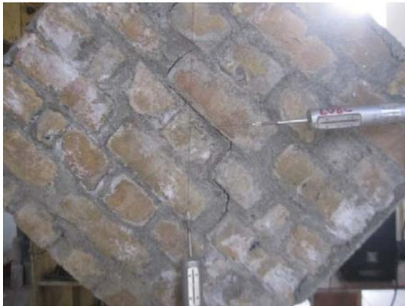
**Fig 9:** Shear (diagonal) cracks of bare prism
