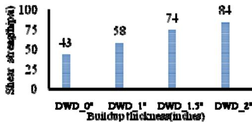
**Fig 8:** Comparison of shear strength of bared & shotcrete double wythe diagonal (DWD) along the buildup thickness.
