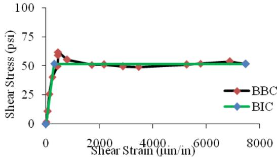
Fig 13: Bi-linear Idealized Curve (BIC) of double wythe shotcrete diagonal prism, (DWD\_1'')
