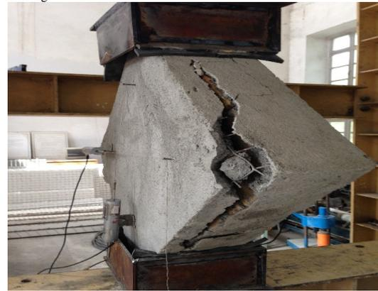
**Fig 10:** Damaged pattern of shotcreted diagonal prism. Comparison of shear & principle tensile strength versus shotcrete thickness
