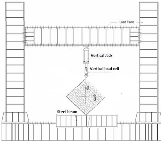
**Fig 3:** Diagonal Tension Test Setup, the numbers (1 & 2) on the specimen represent transducers position.
