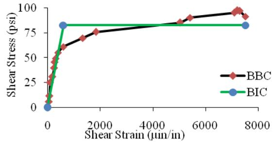
Fig 15: Bi-linear Idealized Curve (BIC) of double wythe shotcrete diagonal prism, (DWD\_2.0'')
