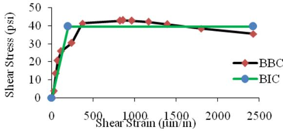
Fig 12: Bi-linear Idealized Curve (BIC) of double wythe diagonal prism, without shotcreting (DWD\_0'')
