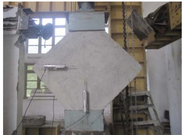
**Fig 6:** Testing of Diagonal Tension (Shear) prisms (ASTM E 519-02)
