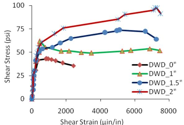
Fig 16: Shear Stress-strain Envelope curves of with & without shotcreting (i.e. 0, 1, 1.5, & 2.0-inches shotcreting)
