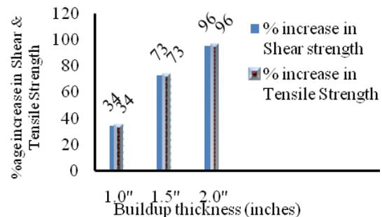
**Fig 11:** Comparison of shear & principle tensile strengths of double wythe diagonal prisms with buildup thickness.
