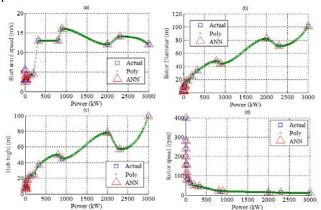
Fig 5: Data results comparisons for HWT based on (a) start wind speed, (b) rotor diameter, (c) hub height, (d) rotor speed.
