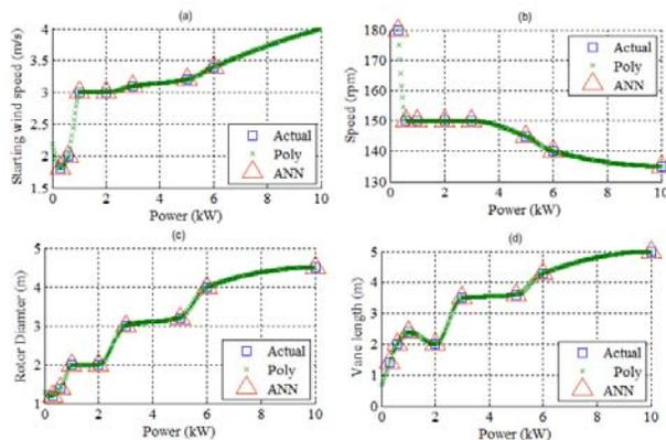
Fig 7: Data results comparisons for VWT based on (a) start wind speed, (b) rotor speed, (c) rotor diameter, (d) vane length
