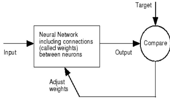
Fig 2: Schematic diagram of ANN concept.
