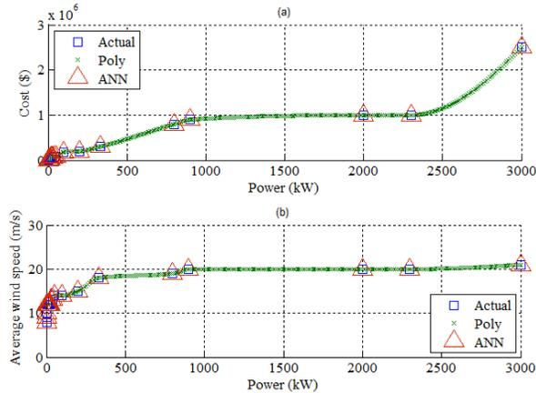
Fig 6: Data results comp.s for HWT based on (a) wind turbine cost, (b)
