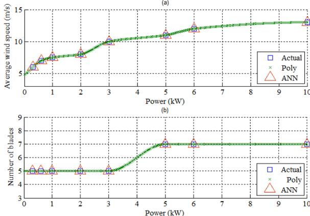
Fig 8: Data results comparisons for VWT based on (a) average wind speed, (b) number of blades.
