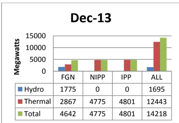
Fig 2: Targeted Increase in Generation Capacity by December 2013 [33]
