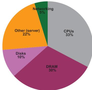
**Fig 5:** Approximate distribution of peak power usage by hardware subsystem in one of Google's data centres (circa 2007). Source: [7].
