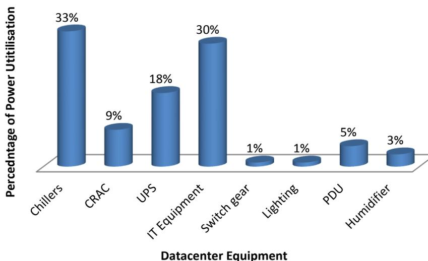
Fig 6: Power Distribution overhead of various Data centre Equipments [22]
