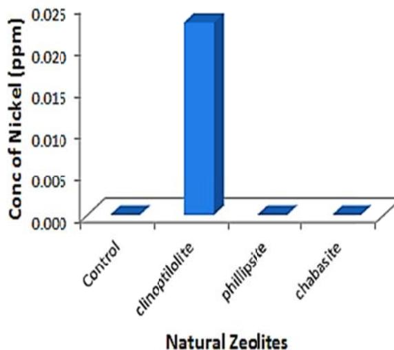
Fig 2: .Nickel concentrations in different zeolites
