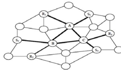
Fig 3: Mesh Configuration in ODMRP.
