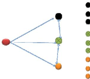
The above diagram shows the result of the bird view model. In mesh topology each and every nodes are interconnected to each other. In first level, there are three possible nodes that covers depend upon the throughput, energy and node behavior from the sink. Likewise, each three nodes further selects the another three nodes and vice versa.
