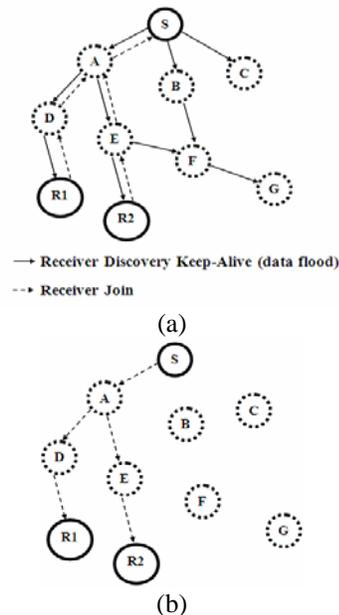
**Fig 1:** ADMR Protocol: (a) Route Discovery, (b) The path Selection.
