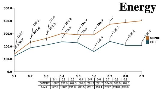
X-axis and Y-axis of the above graph is Time taken in seconds and Number of packets. The above graph shows the energy level of the OMT and OMMRP according to the delivery of the packets. The tabular column shows that the energy of the nodes in OMMRP is high when compared with the OMT [3].
