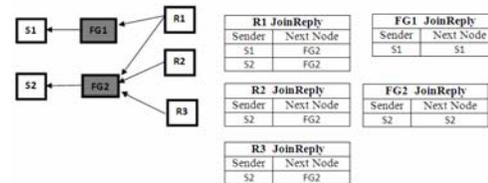
Fig 2: Join- Reply Forwarding in ODMRP.
