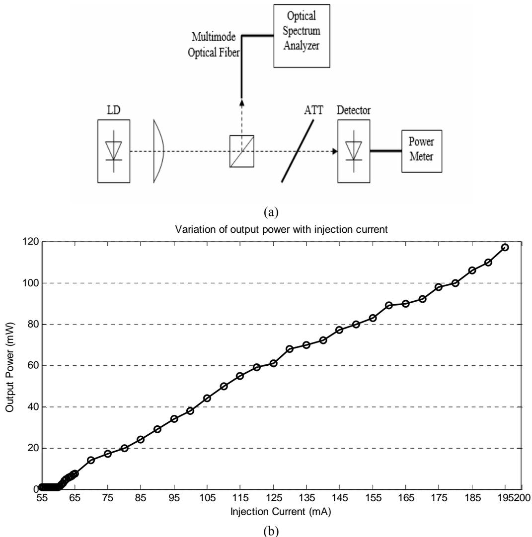
**Fig 9:** (a) Practical setup to measure optical power of laser diodes, (b) Variation of output power with input current injection.
