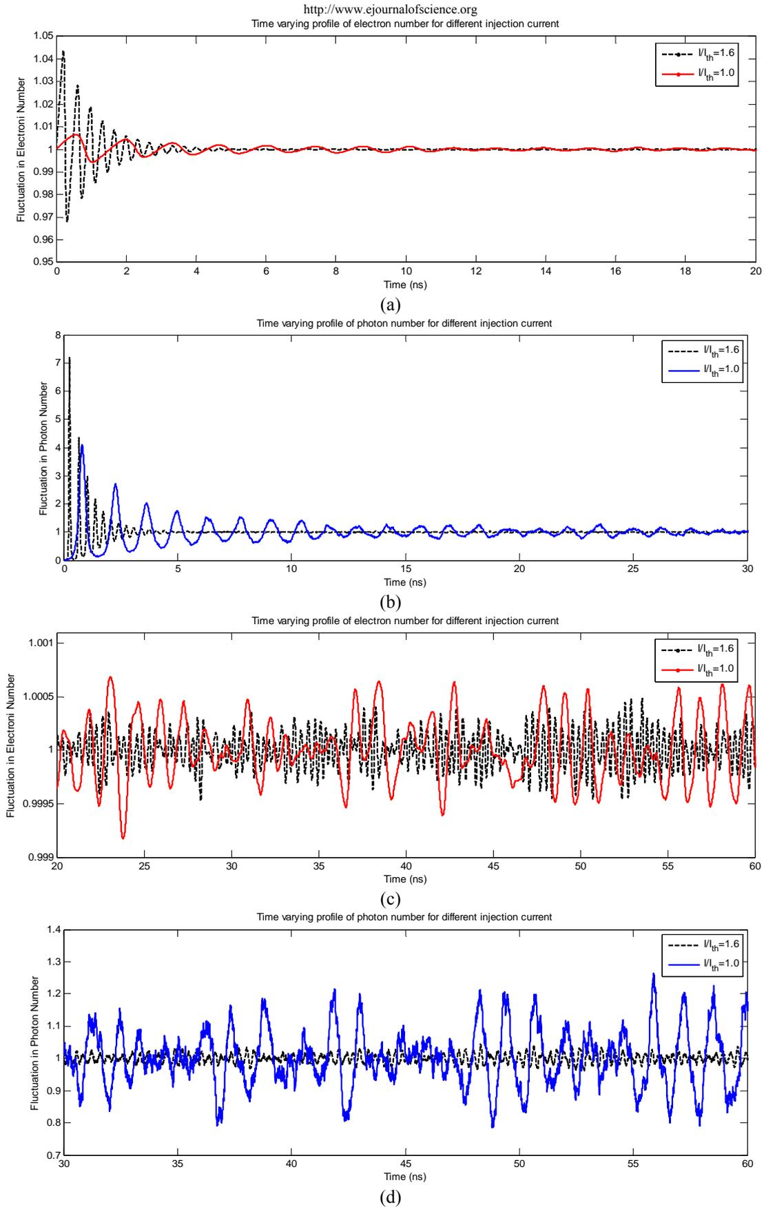
**Fig 3:** Time varying profiles of photon and carrier numbers before and after transient response for two values of injection current ( $I=1.6I_{th}$  and  $I=1.0I_{th}$ ); (a) Time varying profile of the carrier number with transient response. (b) Time varying profile for the photon number with transient response. (c) Time varying profile of the carrier number after transient response dies out. (d) Time varying profile for the photon number after transient response dies out.
