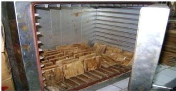
Fig 11: Moisture content specimen tests.
