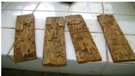
**Fig 25:** specimens test after taken from the ground
