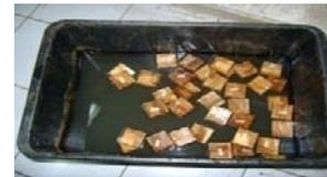
Fig 13: Thickness swelling specimen tests.
