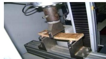
Fig 14: Universal testing machines (instron).
