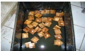
Fig 12: Water absorption specimen tests
