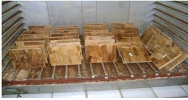
Fig 10: Density specimen tests.
