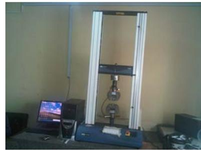
**Fig 1.1:** Tensile test machine (Instron Universal tester series 3369)
