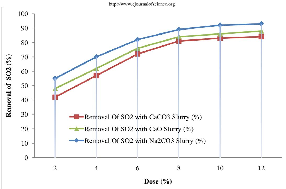
Fig 3: Removal of SO2 with different absorbents at various doses
