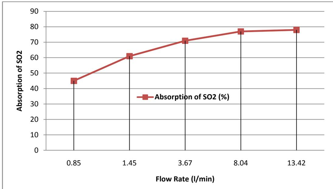
**Fig 2:** %age absorption of SO<sub>2</sub> in water at different flow rates
