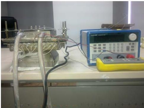
**Fig.4c).** TEG prototype and test platform. This illustrates a TEG prototype built with infrared irradiation as the heat source, water-cooled, and had the same of the rest components as that of Fig -4a and -4b. The variable electronic load and a multi-meter is shown on the r.h.s.
