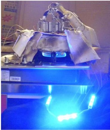
**Fig.4b).** illustrate a type of TEG with the hot-side attached to stove-top, and with the cold-side to a device with running water.
