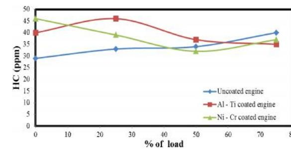
Figure 5: Comparison of Hydrocarbon emission for different loads.
