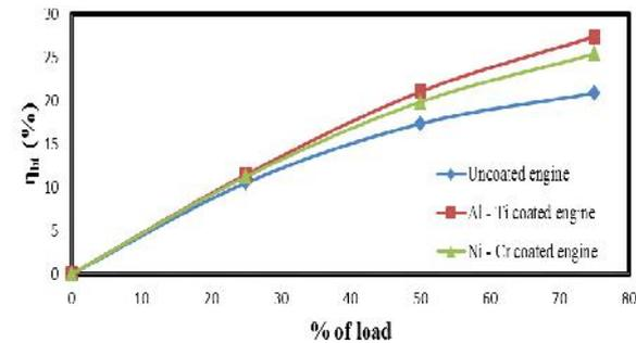
Figure 4: Comparison of Brake Thermal Efficiency for different loads.
