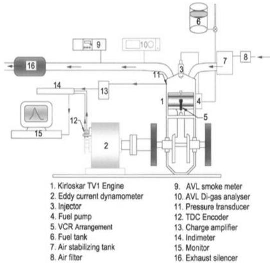
Figure 1: Schematic view of Experimental set-up.
