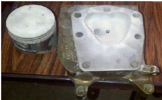
Figure 2: Coated piston and cylinder head
