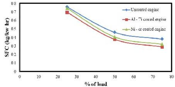
Figure 3: Comparison of Specific Fuel Consumption for different loads.
