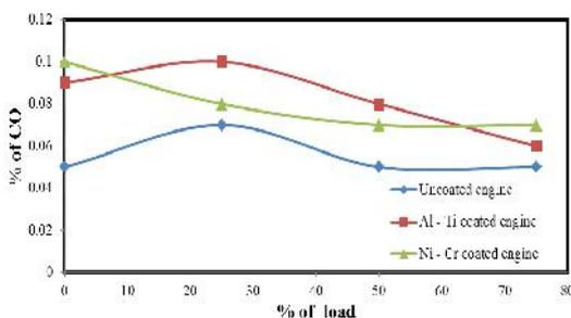
**Figure 7:** Comparison of carbon monoxide emission for different loads.
