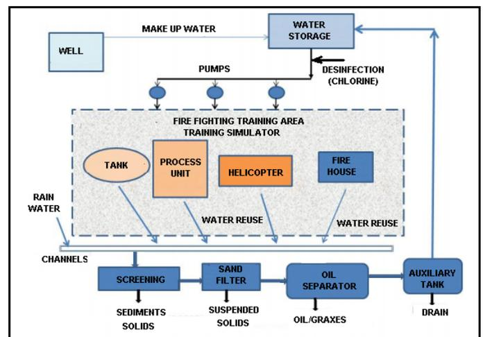
**Fig 2:** Flowchart of the fire fighting installation.
