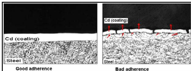
**Fig 3:** Metallography of a cadmium bolt with good and bad adhesion
