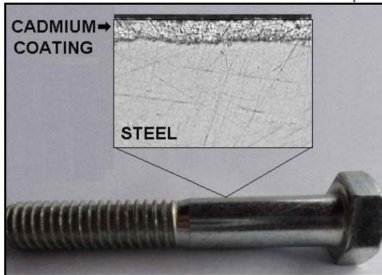
**Fig 2:** Metallographic of a cadmium-coated bolt
