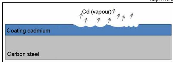
**Fig 4:** Illustration of the vaporization of cadmium coating
