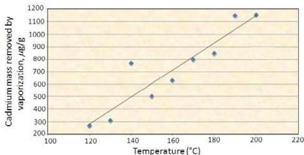
**Fig 6:** Cadmium mass removed by vaporization as a function of temperature
