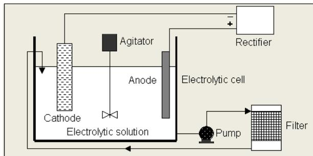
**Fig 1:** Electrolytic cell for deposition of cadmium
