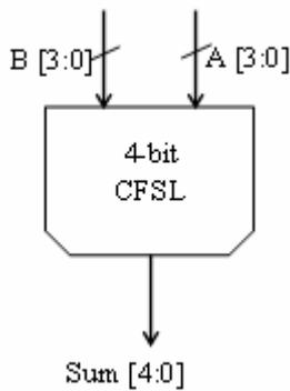
Fig 1: 4-bit Carry free select adder
