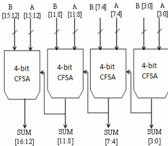
Fig 2: Chain of 4-bit carry free select adder (16-bit adder)
