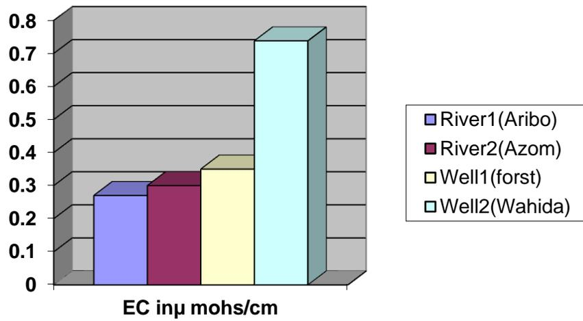
Fig 3: The Electrical conductivity (EC) of Zalingei Water.
