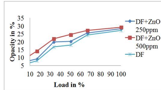
**Fig 6:** The variation of Smoke emission with load for DF and ZnO - DF operation.
