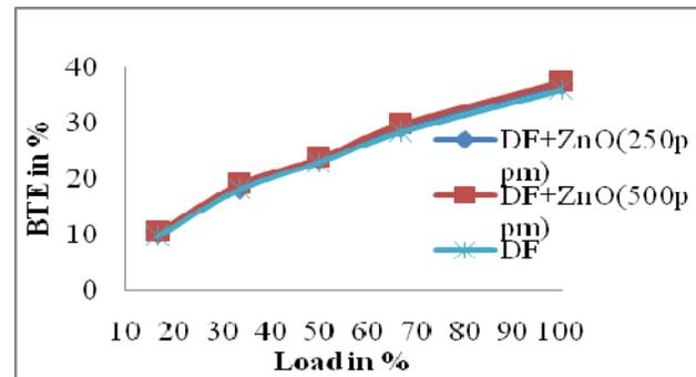
**Fig 7:** The variation of brake thermal efficiency with load for ZnO-DF blends and DF
