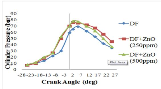
**Fig 3:** The variation of Cylinder Pressure at different Crank Angles for Zinc Oxide Nano particle-DF blends and DF.
