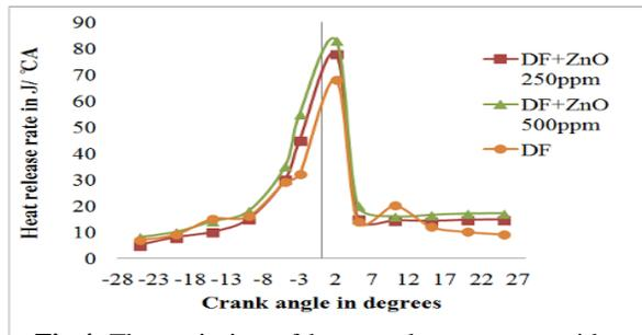
**Fig 4:** The variation of heat release rate with crank angle for ZnO - DF blends and DF.
