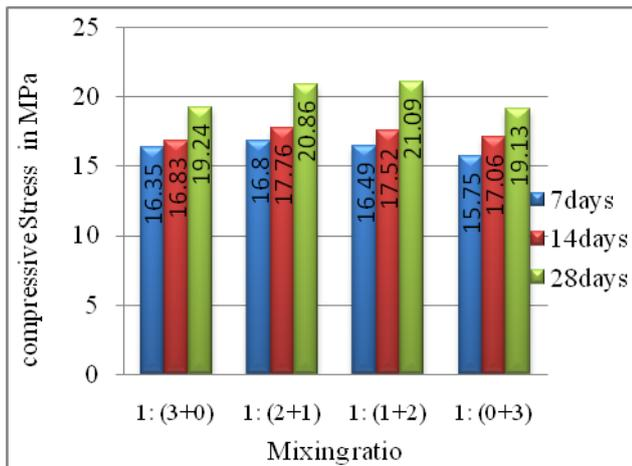
**Fig 2:** Compressive Strength of mortar (1:3) for various mixing ratio
