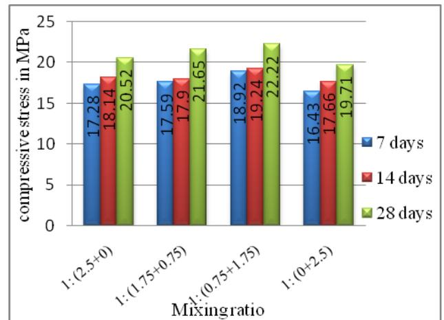
**Fig 4:** Compressive Strength of mortar (1:2.5) of various mixing ratio
