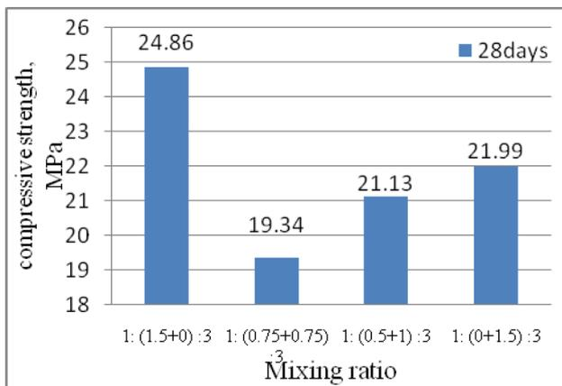
**Fig 7:** Compressive Strength of concrete cylinder of 1:1.5:3 at 28 days
