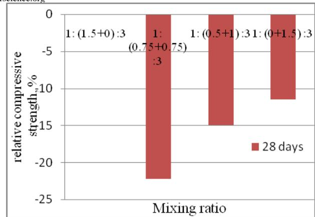
**Fig 8:** Relative strength for different ratio of sand and powder under 1:1.5:3.
