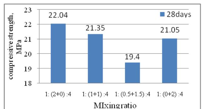
**Fig 5:** Compressive Strength of concrete cylinder of 1:2:4 at 28 days
