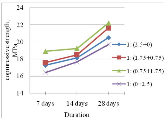
**Fig 3:** Compressive Strength vs. Duration for the mortar of 1:2.5
