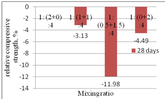
**Fig 6:** Relative strength for different ratio of sand and powder under 1:2:4
