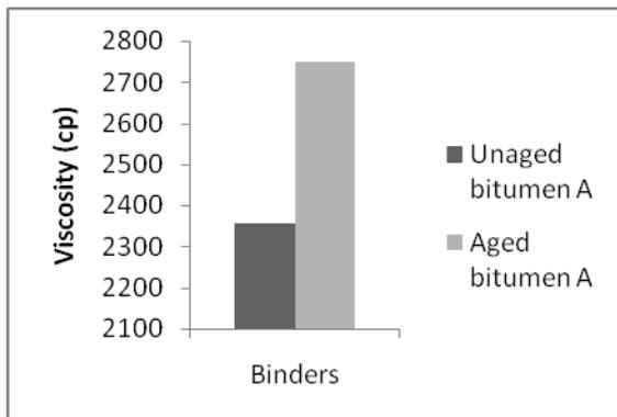
Fig 3: Viscosity trend of bitumen A
