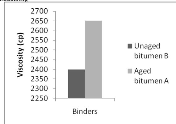
Fig 4: Viscosity trend of bitumen B
