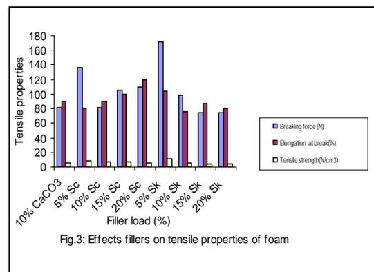
Fig.3: Effects fillers on tensile properties of foam
