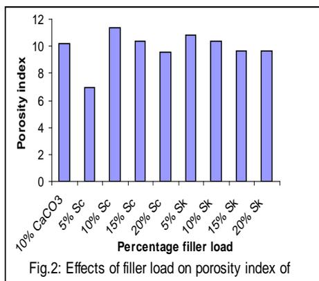
Fig.2: Effects of filler load on porosity index of
