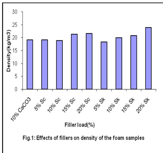
Fig.1: Effects of fillers on density of the foam samples
