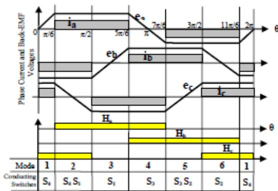
Fig. 1: Current profile , Back EMF , Hall Sensor signals of BLDC motor
