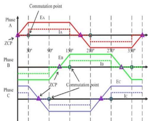
Fig. 3: Position detection of BLDC motor from BEMF
