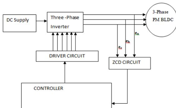
Fig. 2: Conventional position detection of BLDC motor
