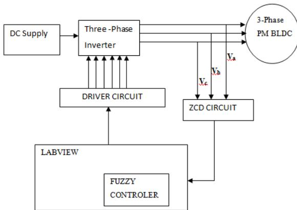
Fig.9: Block diagram of speed control of brushless dc motor using Fuzzy Logic Control in VI.
