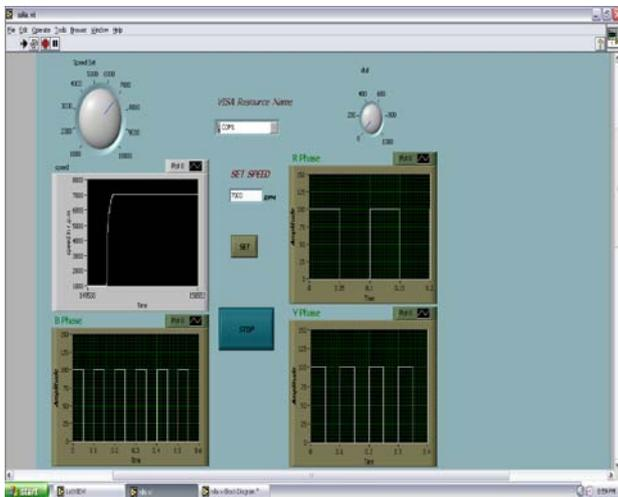
**Fig.12:** Speed output of three-phase PMBLDC motor in Front panel of LABVIEW.
