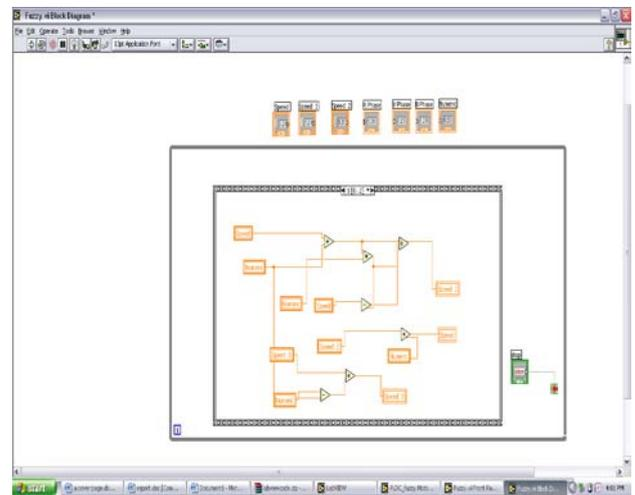
Fig. 7: Stacked sequence-6 Fuzzy control implementation in LABVIEW Programme
