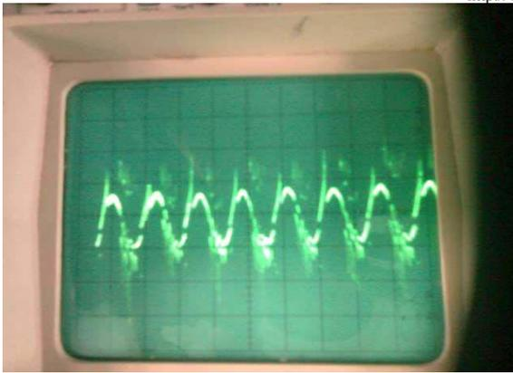
**Fig.11:** Line voltage difference waveform.
