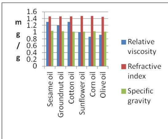
**Fig. (1).** Specific gravity, relative viscosity and refractive index of the six refined edible oils
