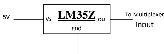
**Figure 2:** LM35z Sensor connection
