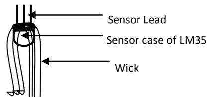
**Figure 3:** Wick constructions for wet temperature sensor
