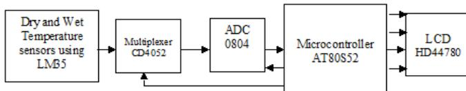
**Figure 1:** The Block Diagram of Automatic Level of Discomfort Index Measurement Instrumentation System
