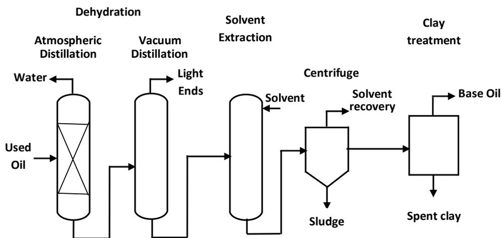
**Fig 1:** Major steps in solvent extraction/clay re-refining process.
