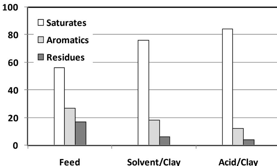
Fig 4: Composition of the feed and re-refined base oils.
