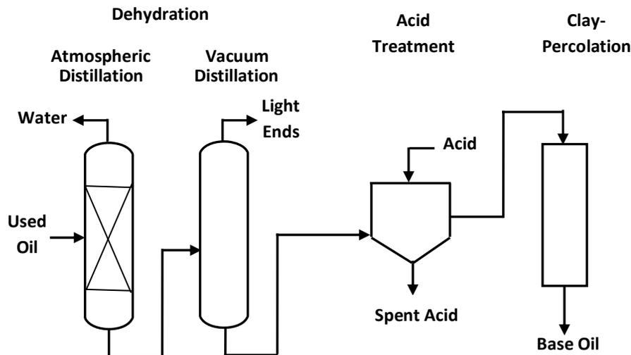
**Fig 2:** Major steps in acid treatment/clay-percolation re-refining process.
