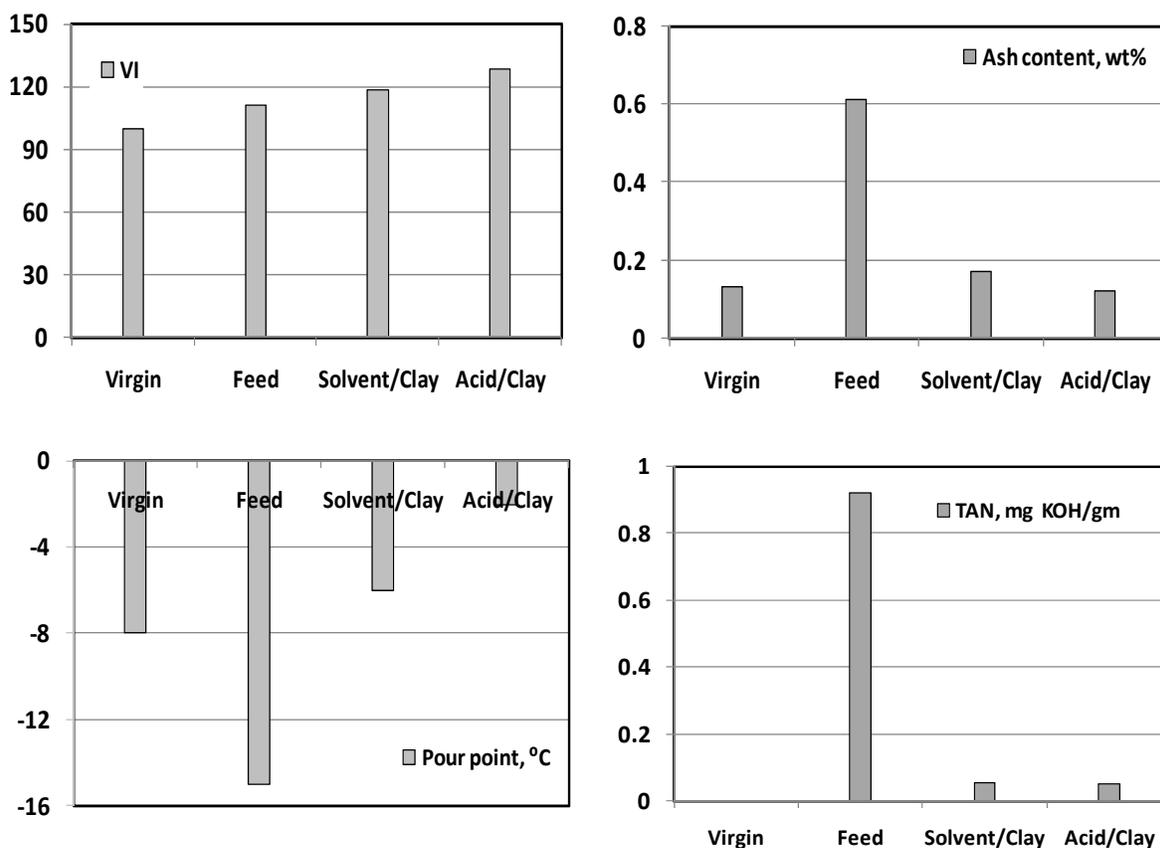
**Fig 3:** Comparison between the properties of re-refined base oil with the virgin and feed oil.
