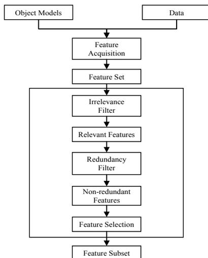
**Fig 4.1:** Feature Selection System Architecture
