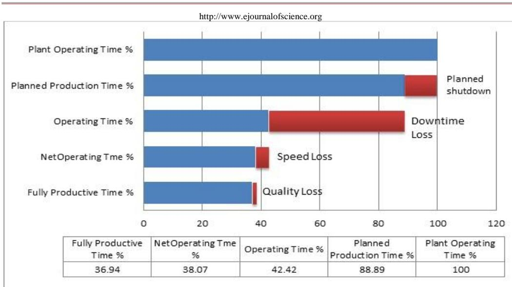
**Figure 8:** Impact of different losses in the reduction of productive time
