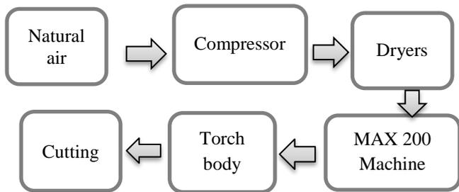
Figure 4: Operation process of CNC cutting
