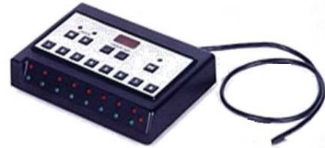
Fig 2: A typical "People Meter" Device for DTH type ROTs
